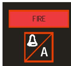
Pressing the "FIRE"/"A" key accepts all the fire alarms that are currently shown in the display. By accepting a fire alarm, the user signals acknowledgement of the fire alarm and that further measures have been introduced. If all fire alarms have been accepted, the field "FIRE" illuminated permanently red.
